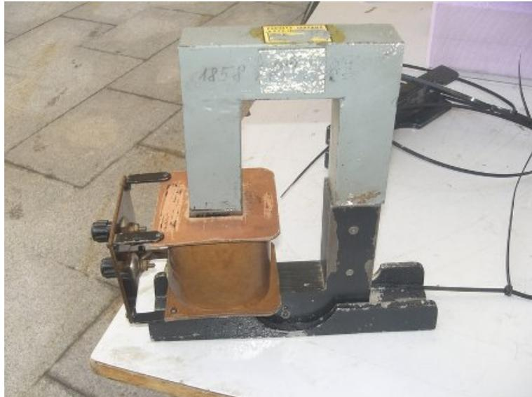
Figure 8: *Transformer core with the coil (primary winding).*
