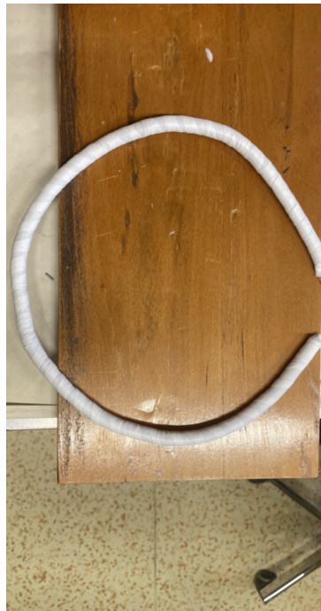
Figure 4.1: New Inner Rogowski Coil Insulated with Teflon Tape.
