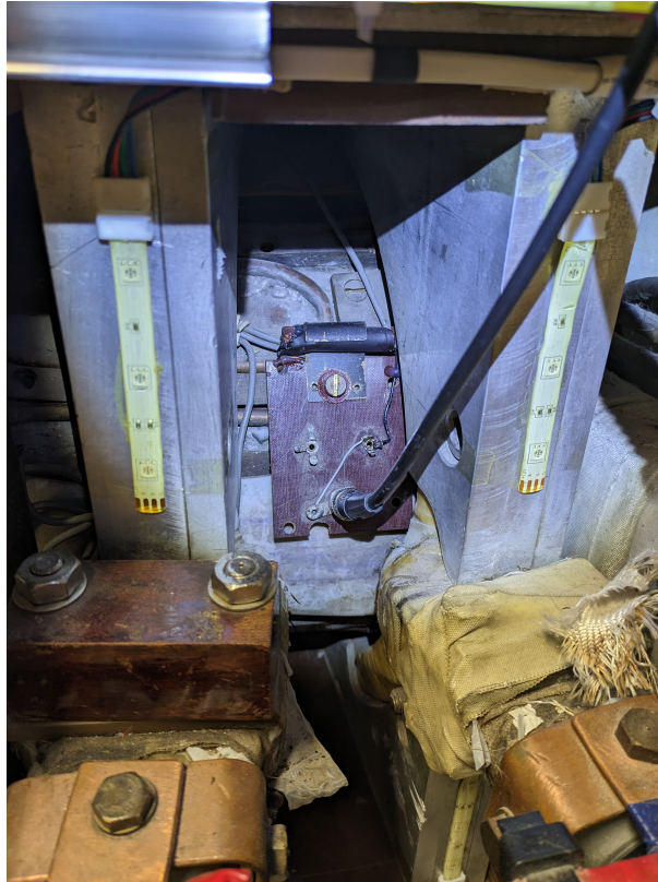
Figure 3.9: Toroidal field measuring coil at GOLEM
