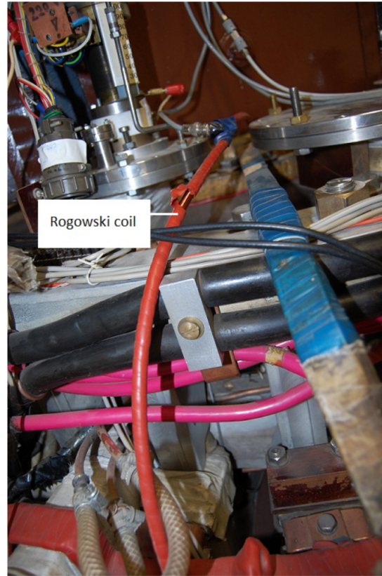
Figure 3.8: Outer Rogowski coil at GOLEM
